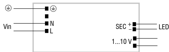
1...10 V diagram Collegamento 1...10 V
